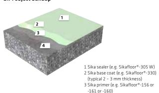
4 Substrate (e.g. concrete or cementitious screed - to be adjusted by BIM user)
