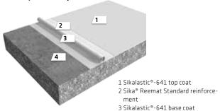
4 Prepared substrate and roof structure (to be adjusted by BIM user)
